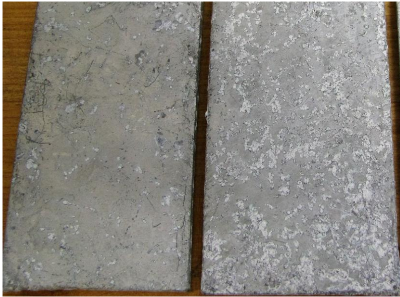
Figure 7 –Test Strip with Factory Pre-treatment (L) Compared to Untreated Galvanized Strip (R)
