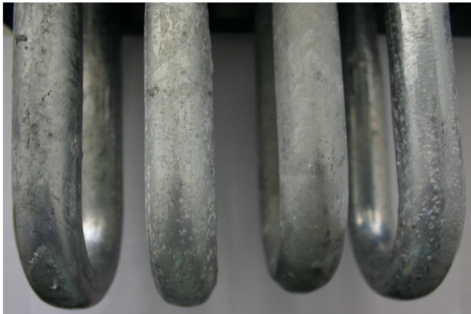
Figure 14 – Photograph of Nano Cooler Coil Sections (from L to R) Test 7 NC-Pre-Treat, NC-Galvanized, Test 8 NC-Pre-Treat, NC-Galvanized
